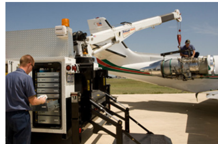
Cessna Citation mobile service unit performing work on the engine of a Cessna Citation Jet
